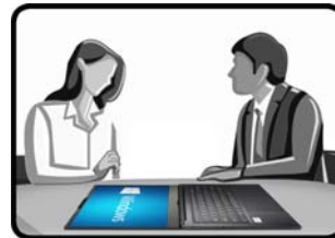
Figure 4 - LCD Panel Open to 180 degrees with Screen Rotated
